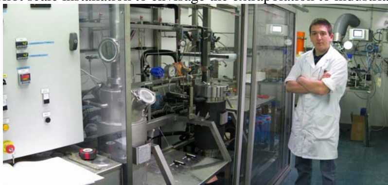
Figure 3: Pilot installation for oxidation of cellulose
